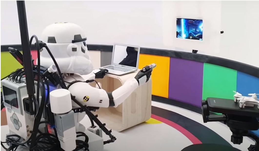
Figure A.18. Setting up an experiment to see if a simple Xzistor agent can derive both Autonomic Stress and Satiation from firing a laser pointer at objects on a screen (effectively Playing a simple game).
