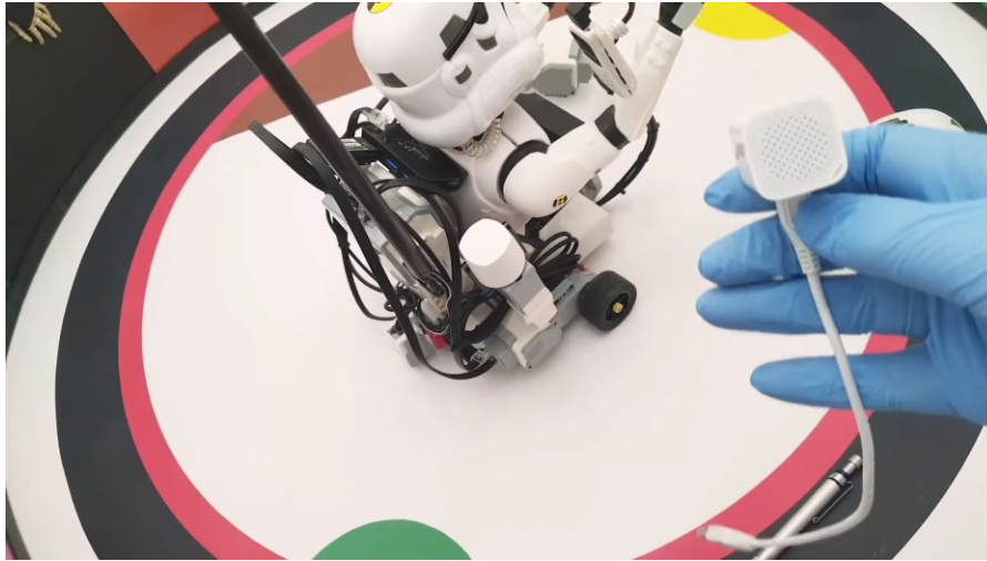
Figure 11. This image shows the small speaker fitted inside the head of the Xzistor robot and connected to the single board computer on the back of the robot that communicates via WiFi with the remote main computer running an instantiation of the Xzistor program.
